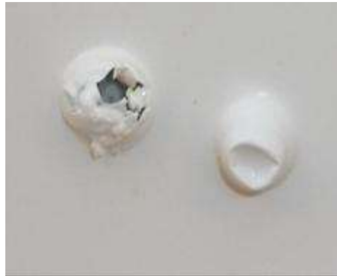
Shunt damage on backsheet
