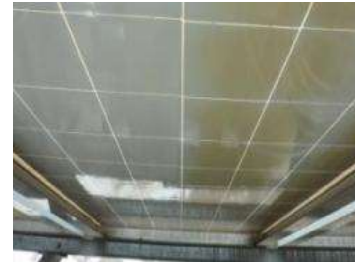
Backsheet air side yellowing
