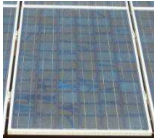
EVA yellowing on cracked cells
